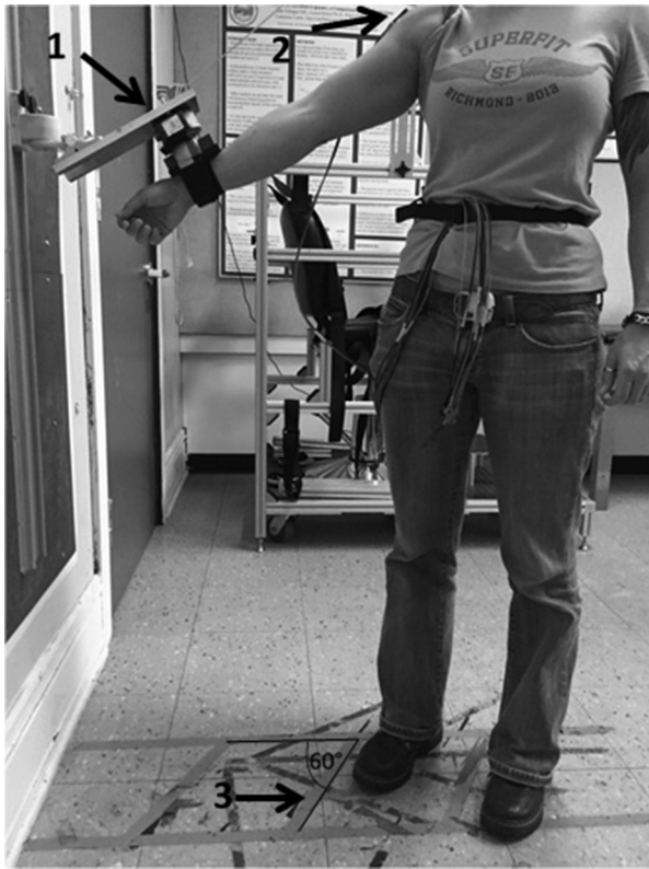
Figure 1 — Experimental setup. (1) Bracket and load cell set flush with forearm at 60° humeral elevation. (2) Middle deltoid electrodes. (3) Floor taping. Tape was placed at 60° from the coronal plane. The subject's feet and pelvis were placed parallel to these lines with the shoulder in line with the bracket. This placed the subject's arm in the scapular plane, approximately 30° anterior to the coronal plane.
