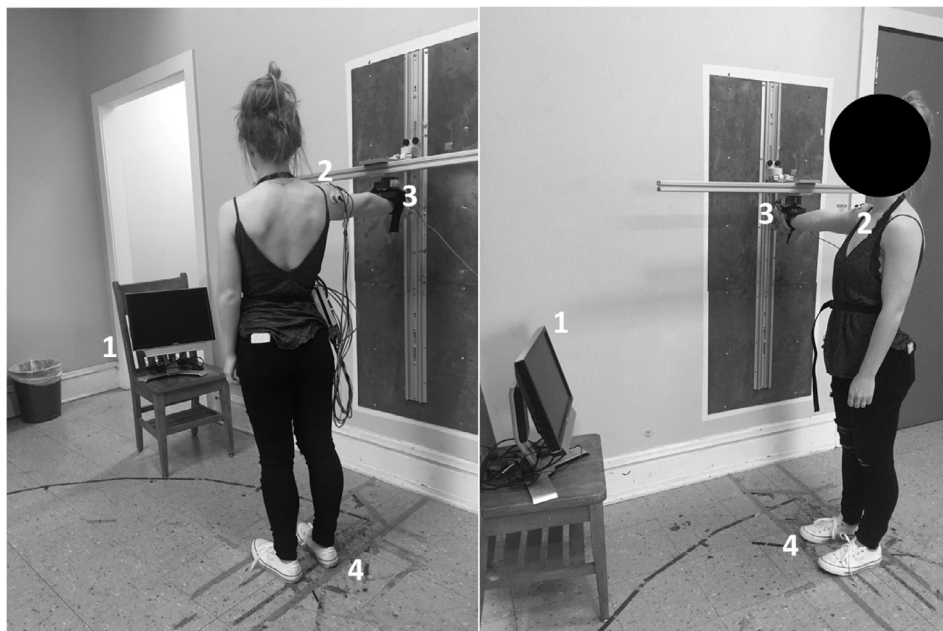
Fig. 1. Experimental setup. (1) Monitor giving feedback on loading rate, (2) surface electrodes on anterior, middle and posterior deltoid, (3) load cell, (4) markings on floor for positioning.
