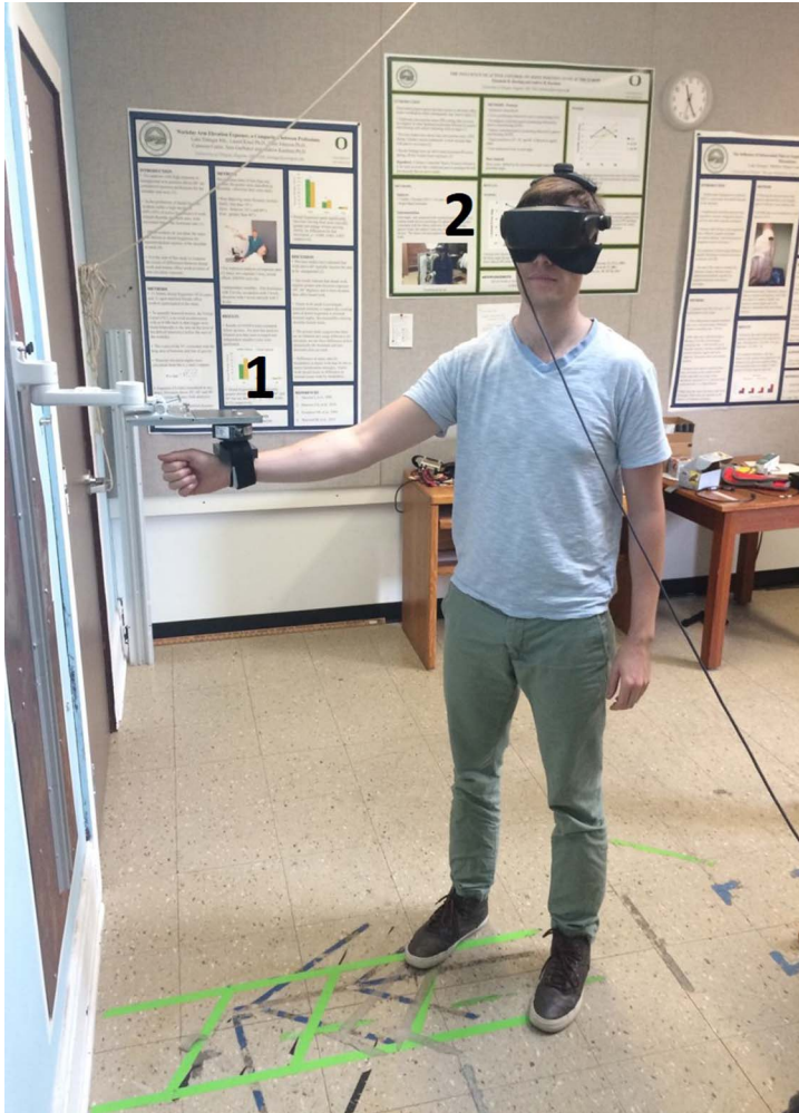
Figure 1 — Experimental setup. Subjects were attached with a Velcro strap at the dominant wrist to a load cell (1) with a head-mounted display (2) providing visual feedback when guiding subjects to a force target. The load cell was mounted to a bracket that could change angles and height on the wall.
